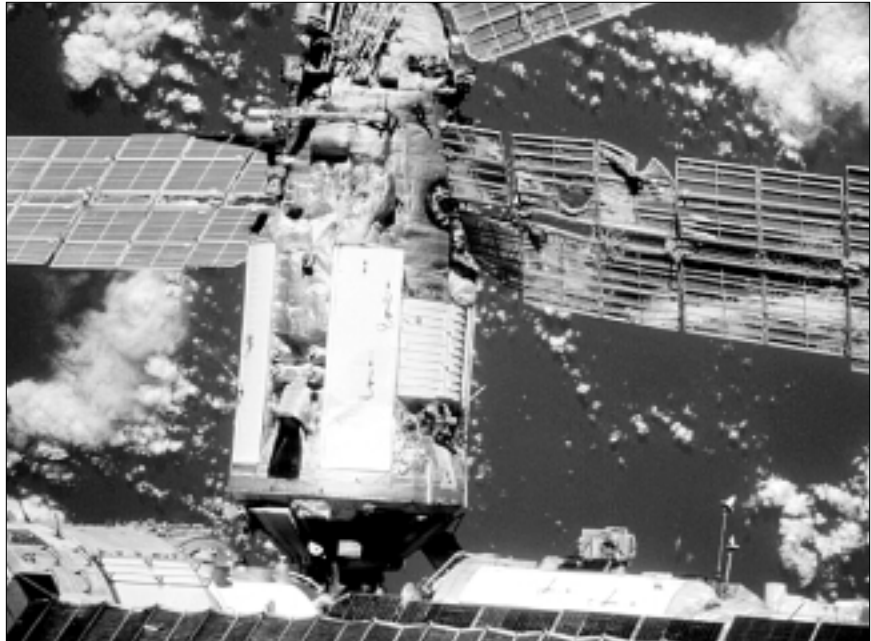
Figure 13: Damage to Spektr module resulting from collision by Progress M-34 cargo vehicle during Mir-23 mission
