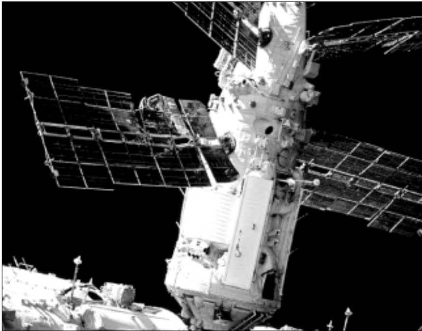
Figure 24: Damage to Spektr module resulting from collision by Progress M-34 cargo vehicle during Mir-23 mission
